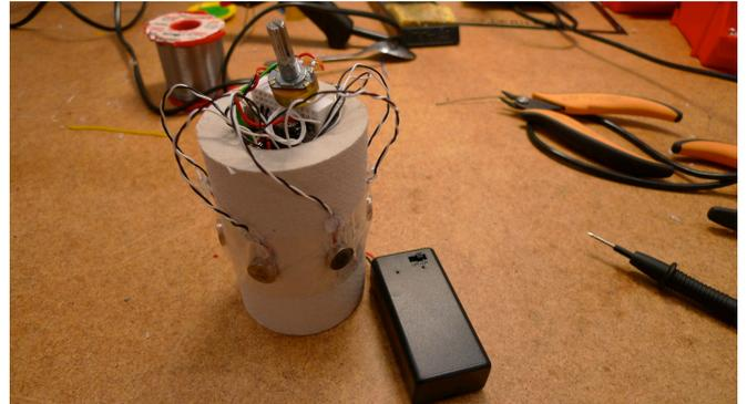
Figure 3: a grip with 7 vibrators, with manual control.
